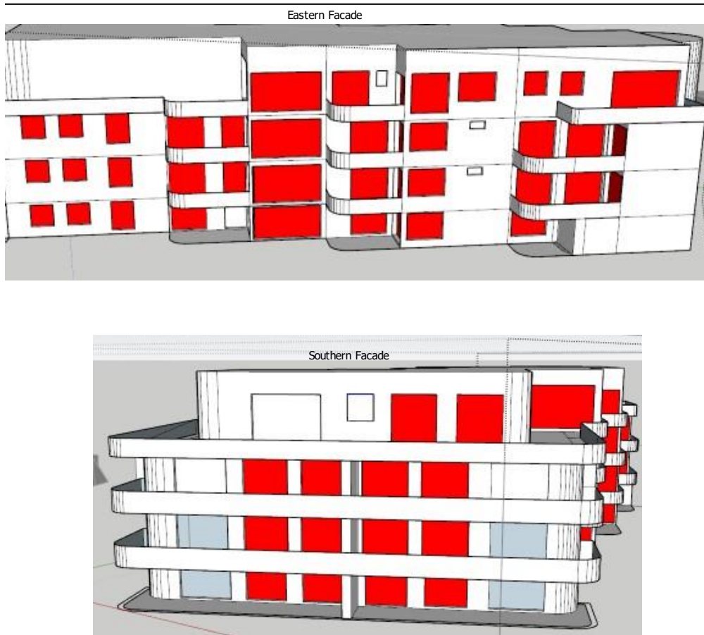
Figure 6 - Apartment Block, Eastern and Southern Façade, Smart Glass Installation Windows
